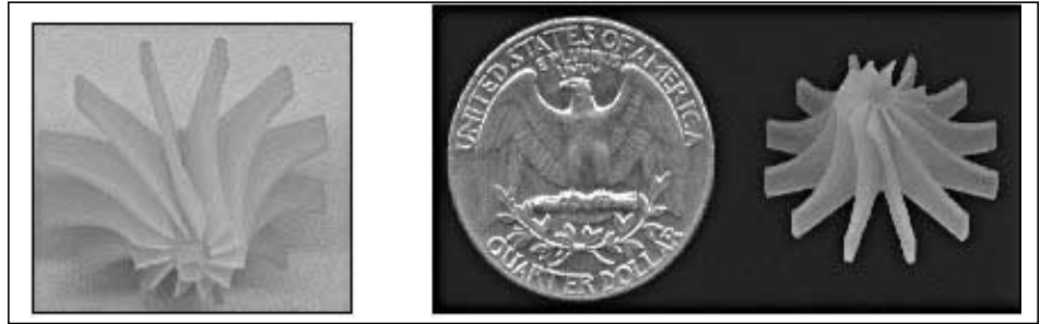
Figure 1. An Inflow Turbine Fabricated by Micro-Stereolithography.
