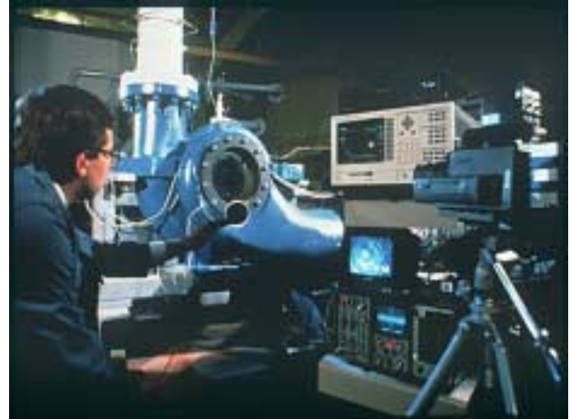
Fig. 2 Viewing cavitation activity in a model pipeline pump impeller.
