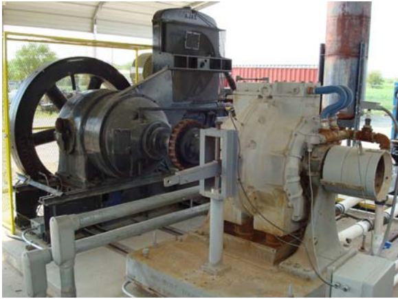
Figure 1: Ajax DP-115 Engine on the Test Stand.
