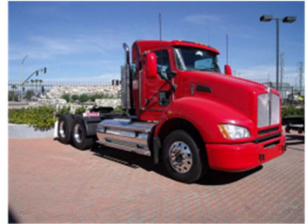
Kenworth T440 2 X 40.5 DGE Rail Mount CNG tanks - 81 DGE
