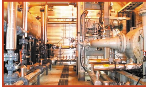
Fig. 1 Field Pilot using Multiphase Pumping (MPP) equipment for improved recovery of organic volatiles resulting from thermal recovery of heavy oil, after MPUR 2003
