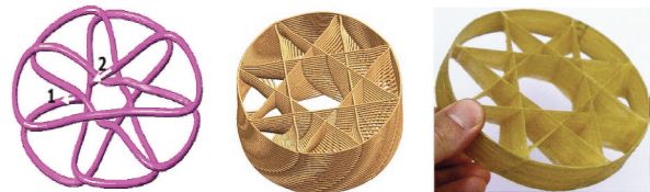
Figure 1. Complete layer for endless fiber winding (left) Computer model wound with single endless fibers (center)
