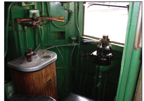
Throttle quadrant (top left), reverser (bottom left) and air brake handle (right).
