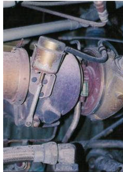
Photo 15: Waste Gate, Series 60
