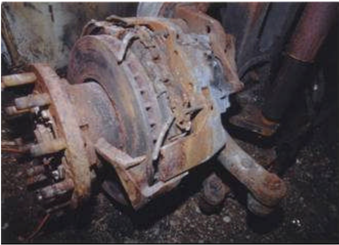
Photo 9: Disc Brake (RH Tag Axle) [Involved]
