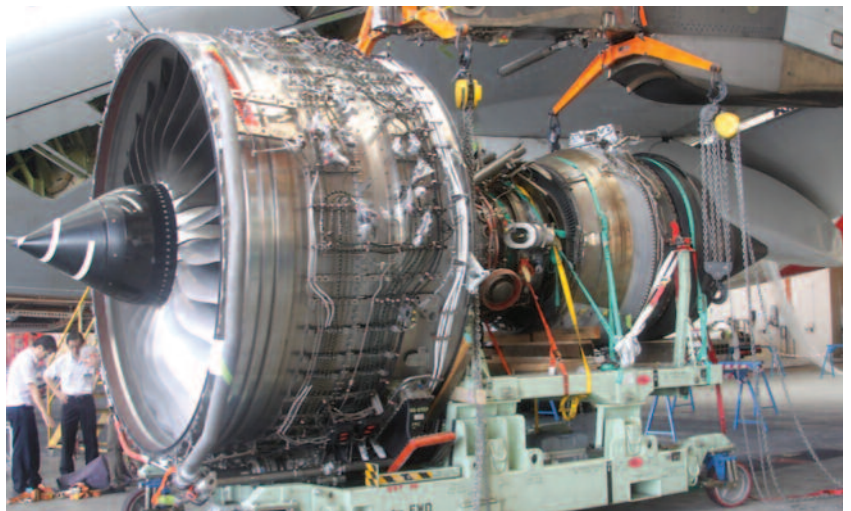
The failed Rolls-Royce Trent 900 engine is removed from a Qantas Airbus A380 [Australian Transport Safety Bureau]
