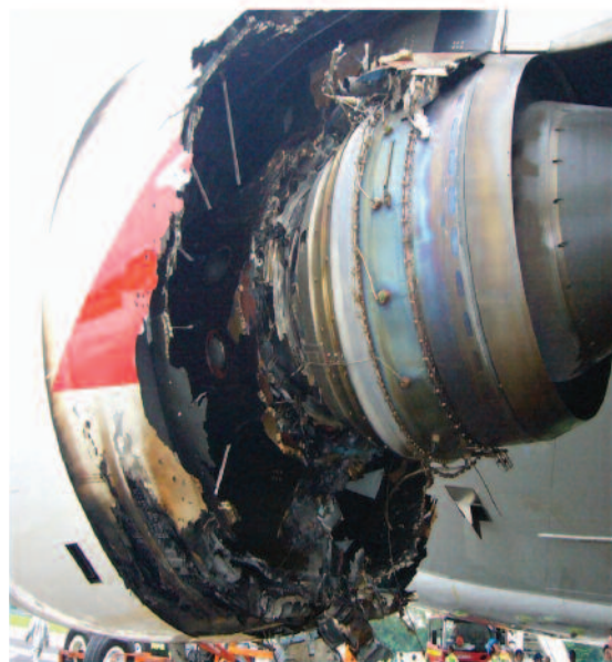
A380 Engine Damage Aft
