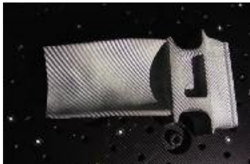
Figure 1: White light scanning fringe pattern being projected onto a 1st stage turbine blade for dimensional data collection.
