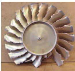
Figure 2. Compressor Rotor Failure.
