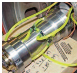
Figure 3. Drive Turbine Housing and Oil-Mist Cooling System.
