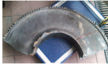
Recovered R-R Trent 900 intermediate pressure turbine disc segment from Qantas A380 Flight QF32. Photo provided by Australian Air Transport Safety Bureau, courtesy of Aviation Week & Space Technology.
