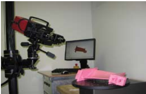
Figure 2 – Representation of the typical setup of a white light scanner being used to collect dimensional data from an injected wax pattern. This data will qualify the wax tooling to be used in the investment casting process.
