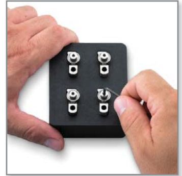
Figure 4: A roller arm fixture assists in assembly. Versus CNC and EDM, there was a 94 percent cost reduction when made with the FDM process. Cost estimate of part pictured:
