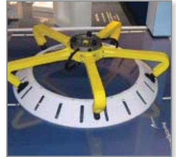
Figure 1: Components for this robotic gripper were first prototyped, then manufactured, using the FDM process
