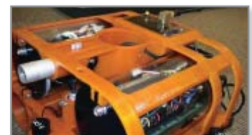
Figures 2 and 3 : University of Central Florida electronics enclosure and the under water vehicle it belongs to. The orange vehicle frame was first prototyped, then manufactured from ABSi using the FDM-based machine
