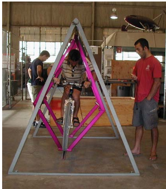
Figure 7: Bike pendulum to determine CG and I_M
