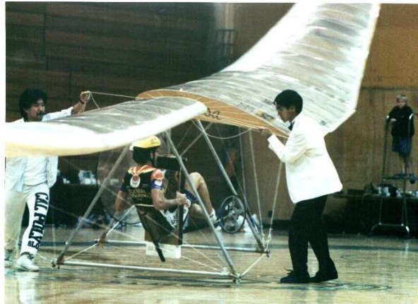
Figure 1: Leonardo III, first successful human powered helicopter
