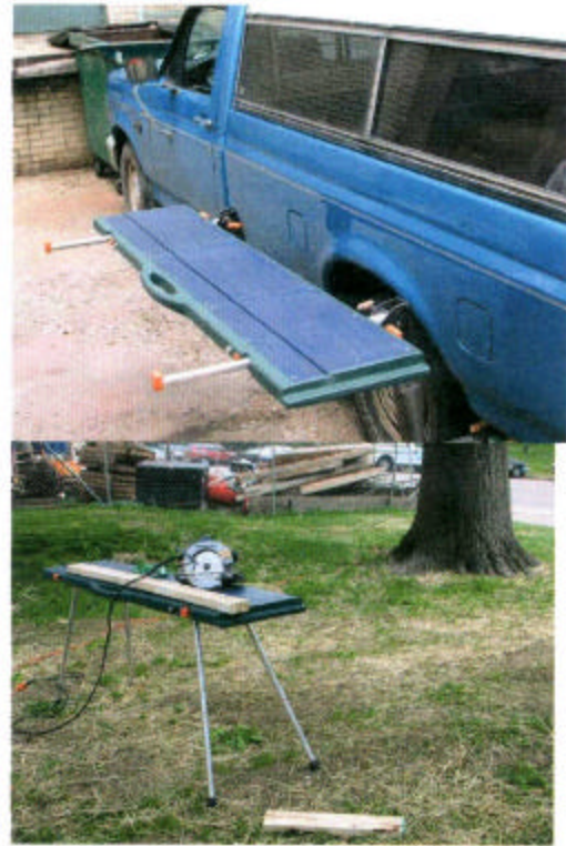
Figure 6: "Sidewinder" worktable for a pickup truck.
