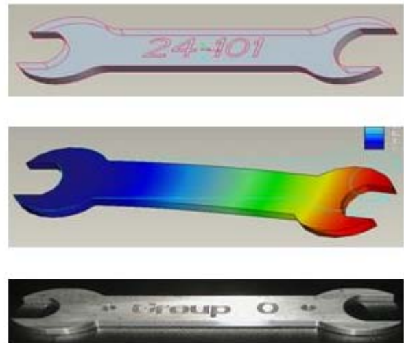
Figure 2: Sequence of modeling, analysis, and manufacturing steps involved in completing the CAE wrench tutorials.
