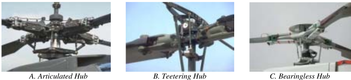
Figure 4: Main Rotor Hub Designs 33
