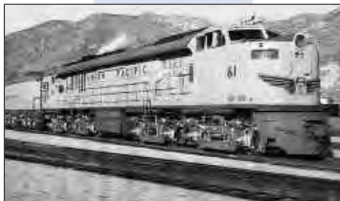
Figure 9. Second Generation GE Gas Turbine Locomotive (4500 HP). 6
