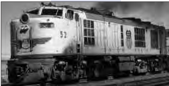
Figure 7. First Generation 4500 HP Gas Turbine Powered Locomotive 2
