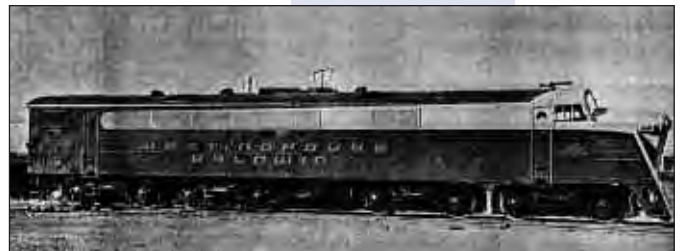
Figure 12. Westinghouse-Baldwin 4000 HP Gas Turbine Locomotive 8
