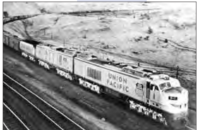
Figure 10. 8500 HP Gas Turbine Powered Train 7
