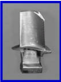
Figure 1. The airfoil tip and a portion of this turbine blade platform came apart due to high cycle fatigue (HCF) during an ultrasonic cleaning operation. The blade material is a single crystal alloy.
