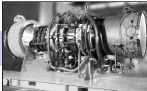
New GE5 Gas Turbine (6 MW range) suitable for small cogeneration plants.
