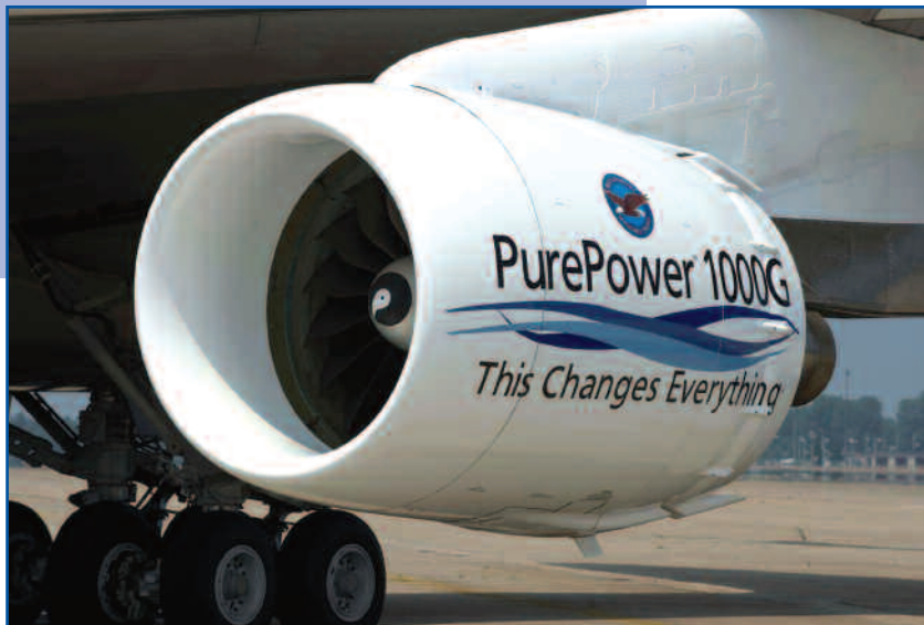
Geared turbofan demonstrator on the wing of Pratt & Whitney's test aircraft.
